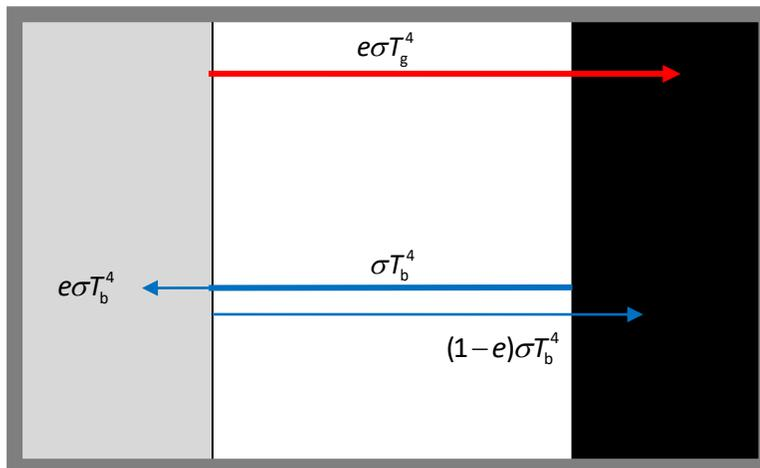
An intensity  $e\sigma T_g^4$  is radiated by the gray body and an intensity  $\sigma T_b^4$  is radiated by the black body. Of the black body radiation incident on the gray body a fraction  $e$  is absorbed. Thus:
